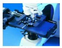
Lower plane of the AS LMD stage. Motor controlled positioning of 4 PCR tubes.
